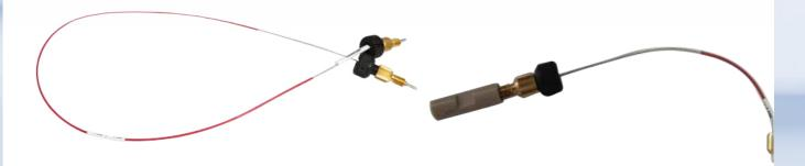
If the fitting is stuck and cannot be removed by hand, try the following: slightly tighten the fitting so it does not leak, connect a column (or a back-pressure tube) to the opposite end of the fitting, and connect the two-port union to the mobile phase line. Start the pump; when the pressure rises to a certain level, loosen the fitting. Under the action of the mobile phase pressure, the fitting will be expelled from the union bore and can then be removed.
