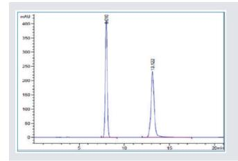
Chromatograhic Conditions: Packing Material: Ultisil CHS C18 (10 µm, 100 Å) Mobile Phase: H2O:CH3OH = 50%:50% Sample: 1. 2, 7-dihydroxynaphthalene, 2. 2, 3-dihydroxynaphthalene Detector: UV, 254 nm Flow Rate: 0.8 mL/min Detector Temperature: 30°C
