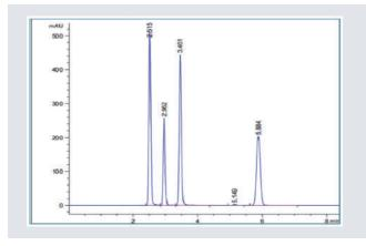
Chromatographic Conditions: Packing Material: Ultisil BHS C18 (10 µm, 120 Å) Part No.: H02755-03100 Mobile phase: H2O:CH3OH=85%: 15% Samples: 1. Uracil, 2. Nitrobenzene, 3. Phenol, 4. Naphthalene Detector: UV, 254 nm Flow rate: 1 mL/min
